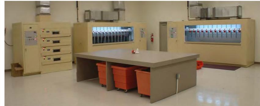
**CURRENT:** The current of each glove/sleeve being tested is continuously monitored by the microprocessor control system. The active current leakage as well as the peak current is displayed on an LCD display both digitally and with a bar graph.
