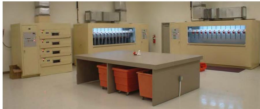
**CURRENT:** The current of each glove/sleeve being tested is continuously monitored by the microprocessor control system. The active current leakage as well as the peak current is displayed on an LCD display both digitally and with a bar graph.
