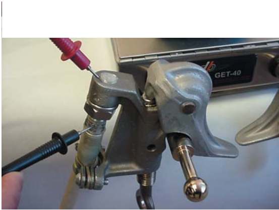
The included 2x2 points test probe can be used to measure specific Personal Grounding Set components (clamp, ferrule or cable).
